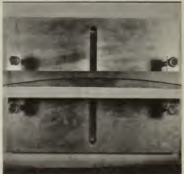
Figure 9 - Film holder. Left: Front view. Note height adjustment screws and lead markers. Right: Plan view. Note curvature of holder and approximate energy scale.
